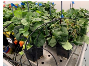
Figure 3.5. After 6 days without irrigation, two of the four strawberry plants on the wireless balance began to wilt. Photo taken on 17 January 2023.
