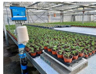
Figure 3.9. A geranium crop on the 30 MHz wireless balance deployed at Staplehurst Nurseries. Photo taken on 2 March 2023.
