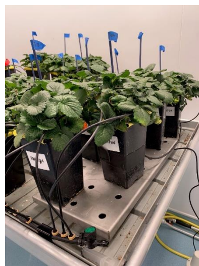
Figure 3.1. The 30 MHz wireless balance in a CE room at NIAB EM. Evaporative water loss from four Malling strawberry plants was recorded continuously from 3 November 2022 to 8 February 2023. Photo taken on 9 December 2022. .
