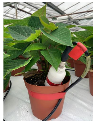
Figure 2.2. An SM150T moisture sensor positioned so that the measuring prongs provided an integrated measure of moisture content across the rooting zone. Photo taken on 3 September 2019.
