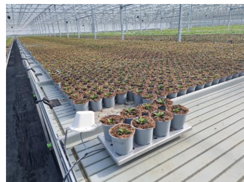
Figure 3.10. An Impatiens crop on the 30 MHz wireless balance deployed at Neame Lea Nursery. Photo taken on 13 March 2023.
