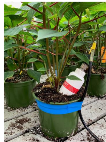
Figure 1.2. An SM150T substrate moisture sensor positioned so that the measuring prongs provide an integrated measure of moisture across the rooting zone. Photo taken on 24 September 2019.
