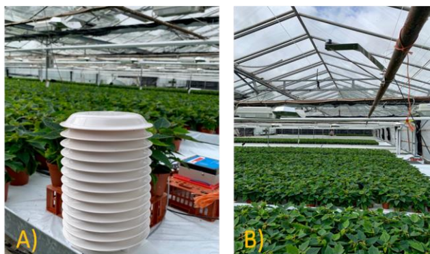
Figure 2.5. A) The air temperature and RH sensor and B) the PAR sensor above the crop used to monitor conditions in the glasshouse at Staplehurst. Photos taken on 12 September 2019.
